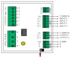
THE JUMPER MUST BE CONNECTED ONLY ON THE 1ST AND LAST XMETER 96 OF THE SERIES (RS485) To connect bridge on jumper remove the safety from all the terminals and only after the silk-screened back.
