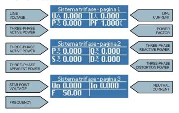
From these pages by using the keys RIGHT and UP it is possible to enter the detail of the remaining measures. To enlarge the measurement press the RIGHT key again.
