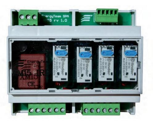
The X-Meter counts 4 ON-OFF output activators to manage 4 outputs with 24Vac/Vdc maximum voltage and 100mA maximum current.
