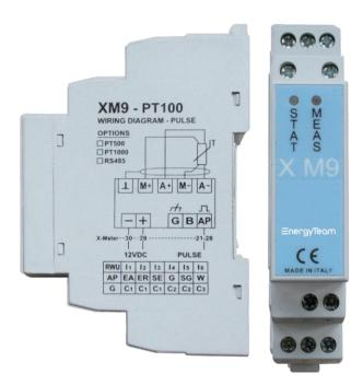
XM9 collects temperature data using PT100, PT500 or PT1000 probes and converts the values in pulsed output with 0 to 5Hz frequency. The minimum value on the measurement scale will imply a 0Hz (0 pulses per second) output pulse frequency while the full scale will mean a 5 Hz (5 pulses per second) output pulse frequency. The probes that can be used may be 2, 3 or 4 wires, even with shielded cable. There also is a 2.5 KV galvanic isolation between the inputs and the other connections.
