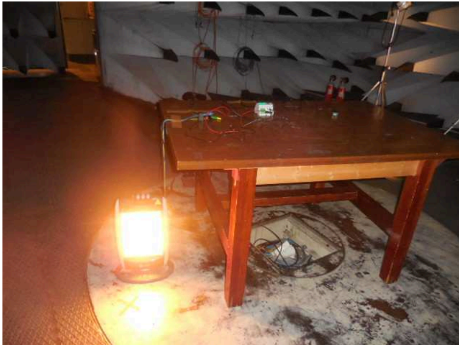
Photo of test setup for Radiated Disturbance, from 30 MHz to 1 GHz
