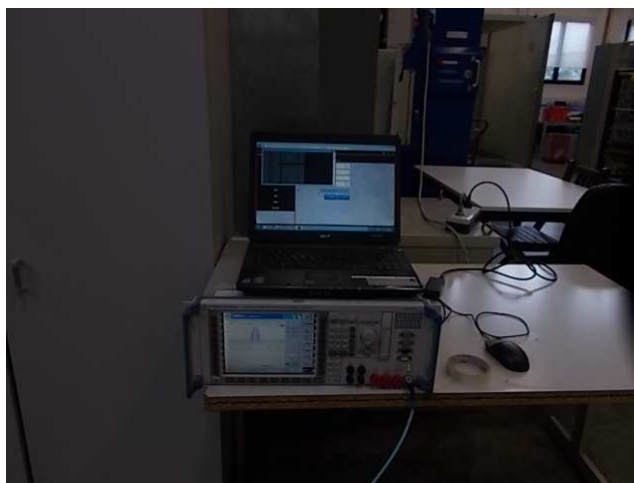
GSM link with CMU200 and ping with PC.
