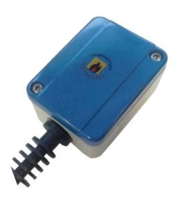
4 wires PT100 probe with sensor protected by an anodized aluminium finned element. Cables housed in a plastic IP65 box.
