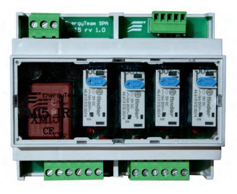
The X-Meter counts 4 ON-OFF output activators to manage 4 outputs with 24Vac/Vdc maximum voltage and 100mA maximum current. These outputs must be interfaced with an XM15 module to manage standard loads in a 220Vac single phase network.
