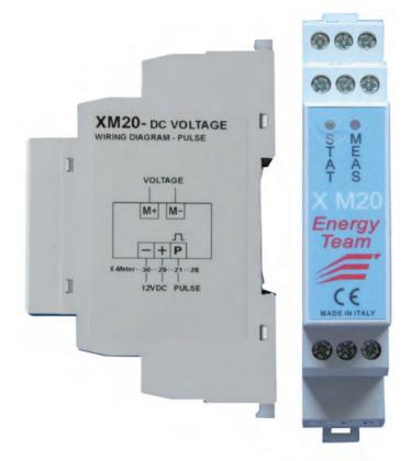
The XM20 device reads a continuous analogical voltage signal up to 1000VDC and converts it into a 0-5 Hz pulsed signal compatible with the standard input signals for CM2 Solar or XRWU GOLD/X-Meter. Guaranteed precision of 0.5% of full scale.
